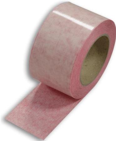
Winflex® Optima – Sealing tapes for abutment joints on windows and exterior doors. Corresponds to RAL installation guidelines and DIN 4108-7. Winflex® Optima allows transverse stretching for optimal absorption of structural movement.
