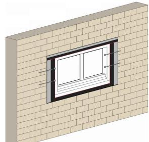
whereby the length exceeds by the side joint width by +0.5 cm at the left and right in the lintel area and the lengths are fitted at the sides with 0.5 cm excess at the top and the joint width of the parapet + 0.5 cm at the bottom. There is no need to differentiate between the room and outdoor sides and there is no risk of confusion. Winflex<sup>®</sup> TriSave eco is butt jointed at the corners.
