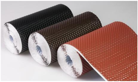
Rooflex® XL es has a calotte embossed surface, therefore it permits optimal attachment on the desired point to conform to the desired shape. The metal surface is weather proof and UV resistant. For optimal handling, the adhesive layer is covered with a siliconised, tear proof, divided, and overlapping plastic foil.
