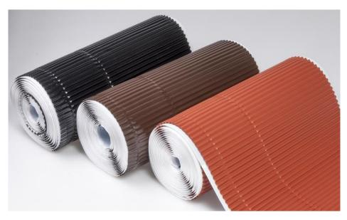
better handling, Aluflex<sup>®</sup> es has two pre-determined folding points, approximately 35 and 115 mm from the edge. This asymmetrical preparation of the material permits optimal attachment after the required material has been cut off in the exact size needed. For optimal handling, the adhesive layer is covered with a siliconised, tear-proof, divided and overlapping plastic foil.
