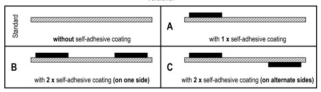
Self-adhesive coating up to 150 mm foil width 20 x 1 mm butyl rubber up to 200 mm foil width 40 x 1 mm butyl rubber
