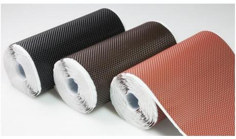
Rooflex® es has a calotte embossed surface, therefore it permits optimal attachment on the desired point to conform to the desired shape. The metal surface is weather proof and UV resistant. For optimal handling, the adhesive layer is covered with a siliconised, tear proof, divided, and overlapping plastic foil.
