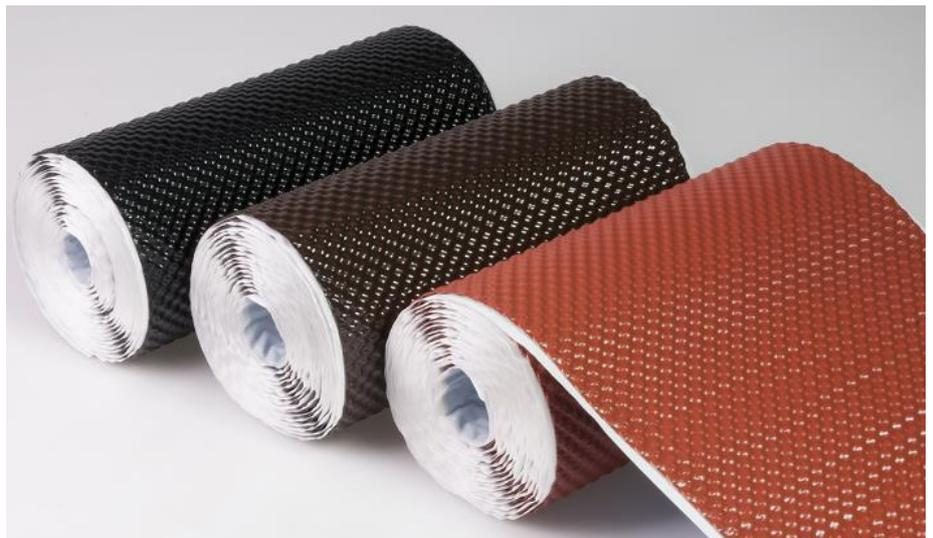
Rooflex® XL es has a calotte embossed surface, therefore it permits optimal attachment on the desired point to conform to the desired shape. The metal surface is weather proof and UV resistant. For optimal handling, the adhesive layer is covered with a siliconised, tear proof, divided, and overlapping plastic foil.
