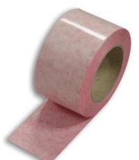
Winflex® Optima – Sealing tapes for abutment joints on windows and exterior doors. Corresponds to RAL installation guidelines and DIN 4108-7. Winflex® Optima allows transverse stretching for optimal absorption of structural movement.
